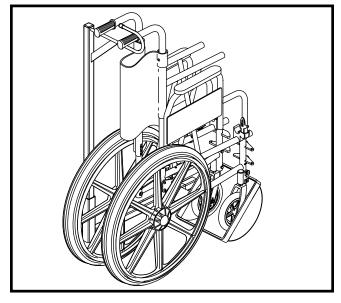
6. Lift the folded wheelchair and place the front caster wheels in the front caster bracket. Secure the wheelchair handles over the vertical hook post.
