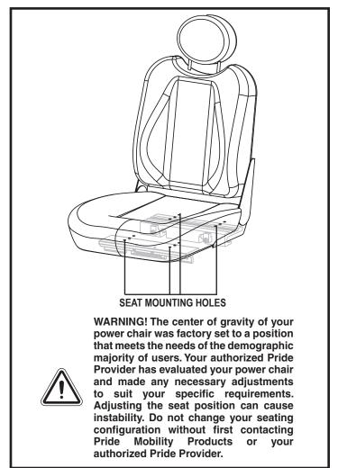
**Figure 9. Seat Position Adjustment**
