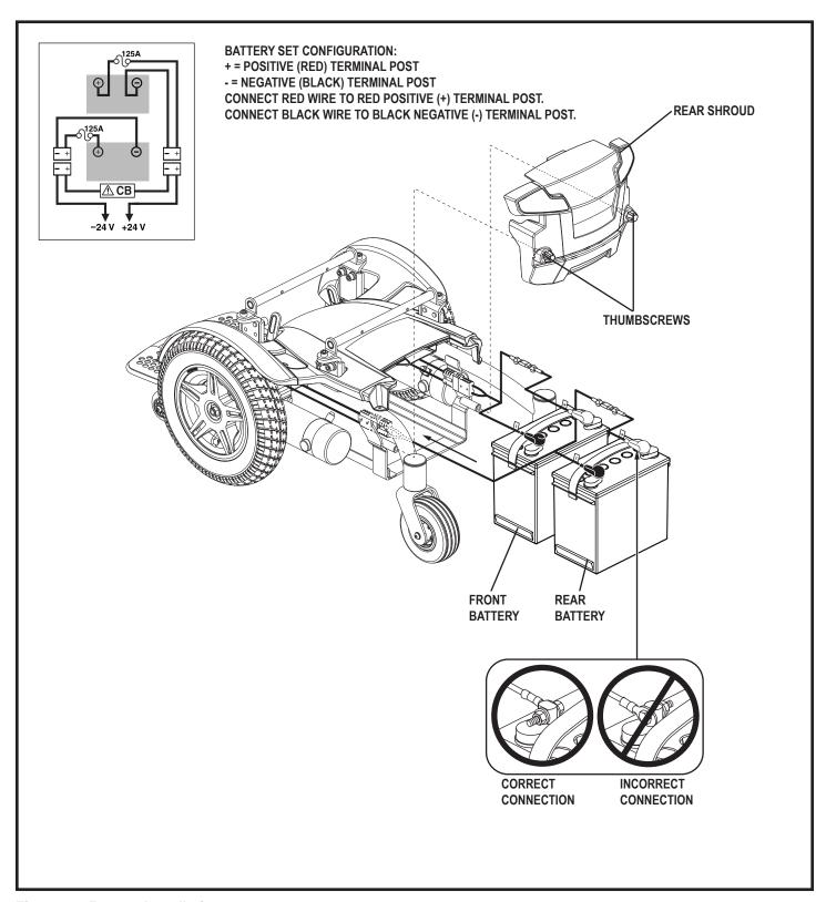
Figure 20. Battery Installation
