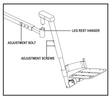
Figure 15. Heavy Duty Drop-in Leg Rests
