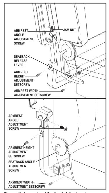
Figure 10. Armrest and Seatback Adjustments
