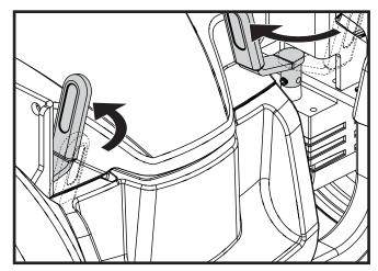
Figure 4. Drive Mode (Drive Engaged)
