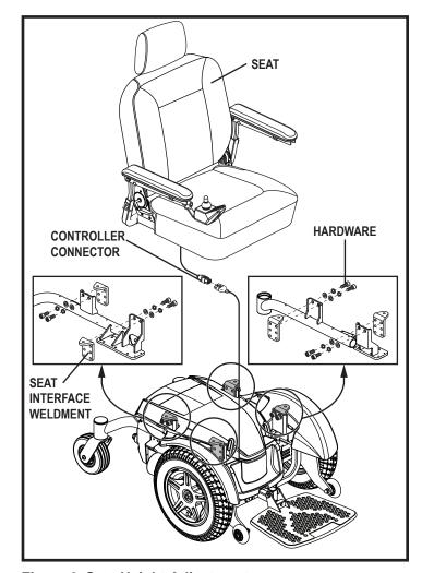
Figure 8. Seat Height Adjustment
