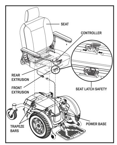
Figure 6. Seat and Controller Assembly
