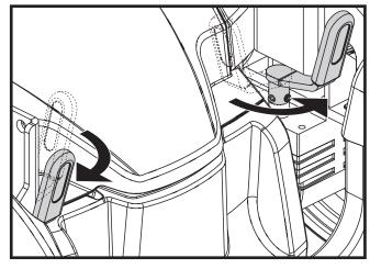
Figure 5. Freewheel Mode (Drive Disengaged)
