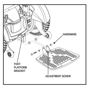
Figure 12. Foot Platform Angle Adjustment
