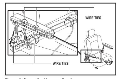
Figure 7. Controller Harness Routing
